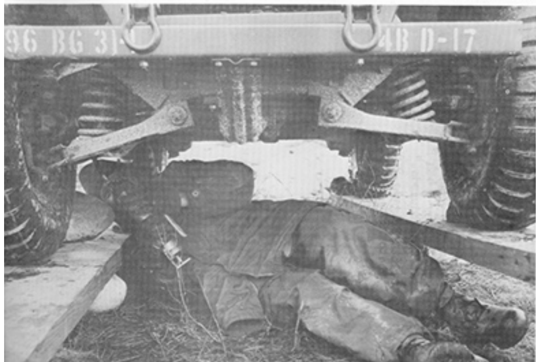
Grease pit in the field
